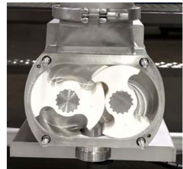
Pump rotor detail shown with cover plate removed.
