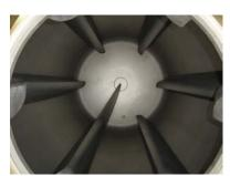
Contoured wing design allows for hard or gentle tumbling action during defrost with optimal flow conditions for ideal energy transfer (heat or cold).
